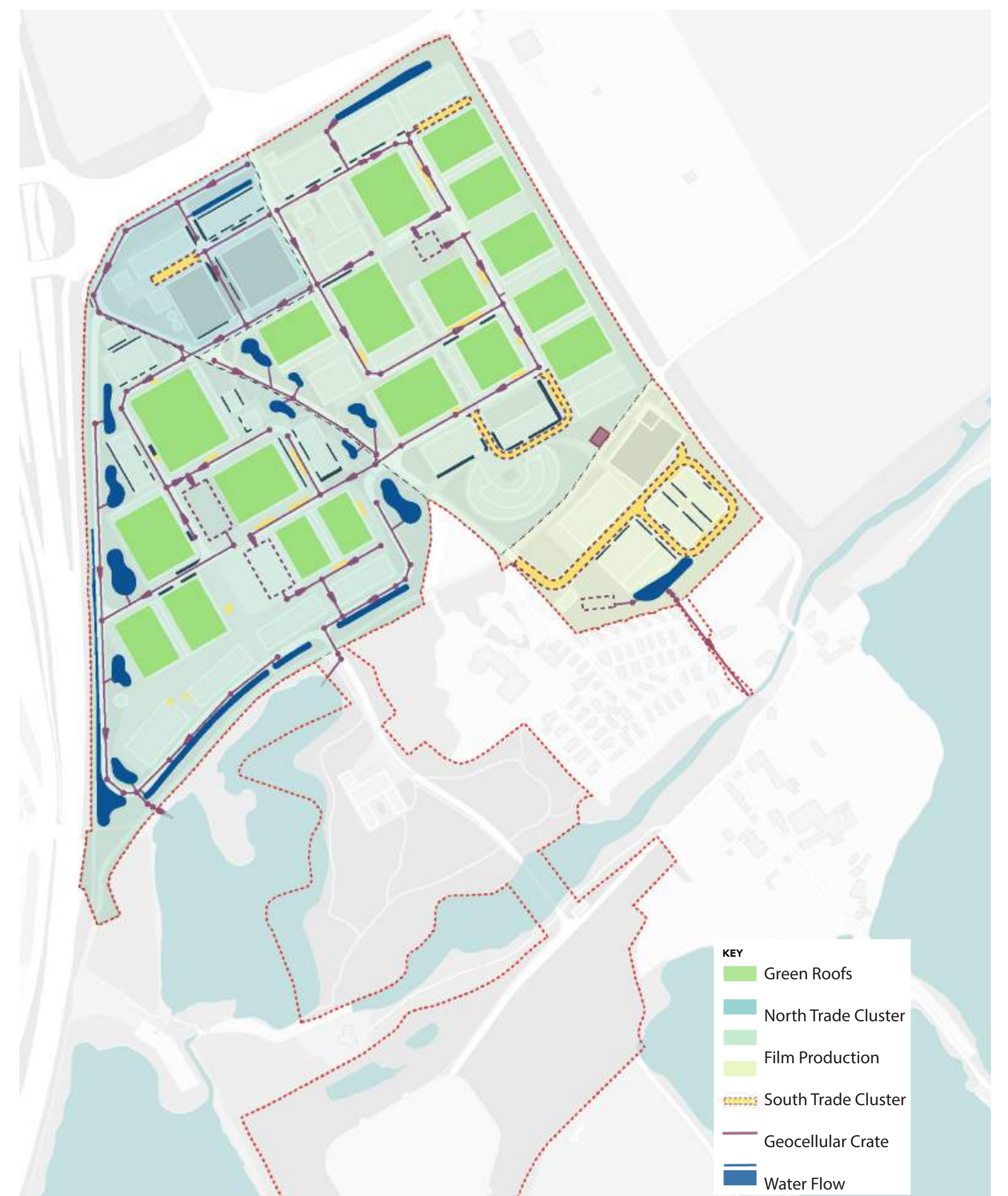
Diagram showing the site drainage plan
