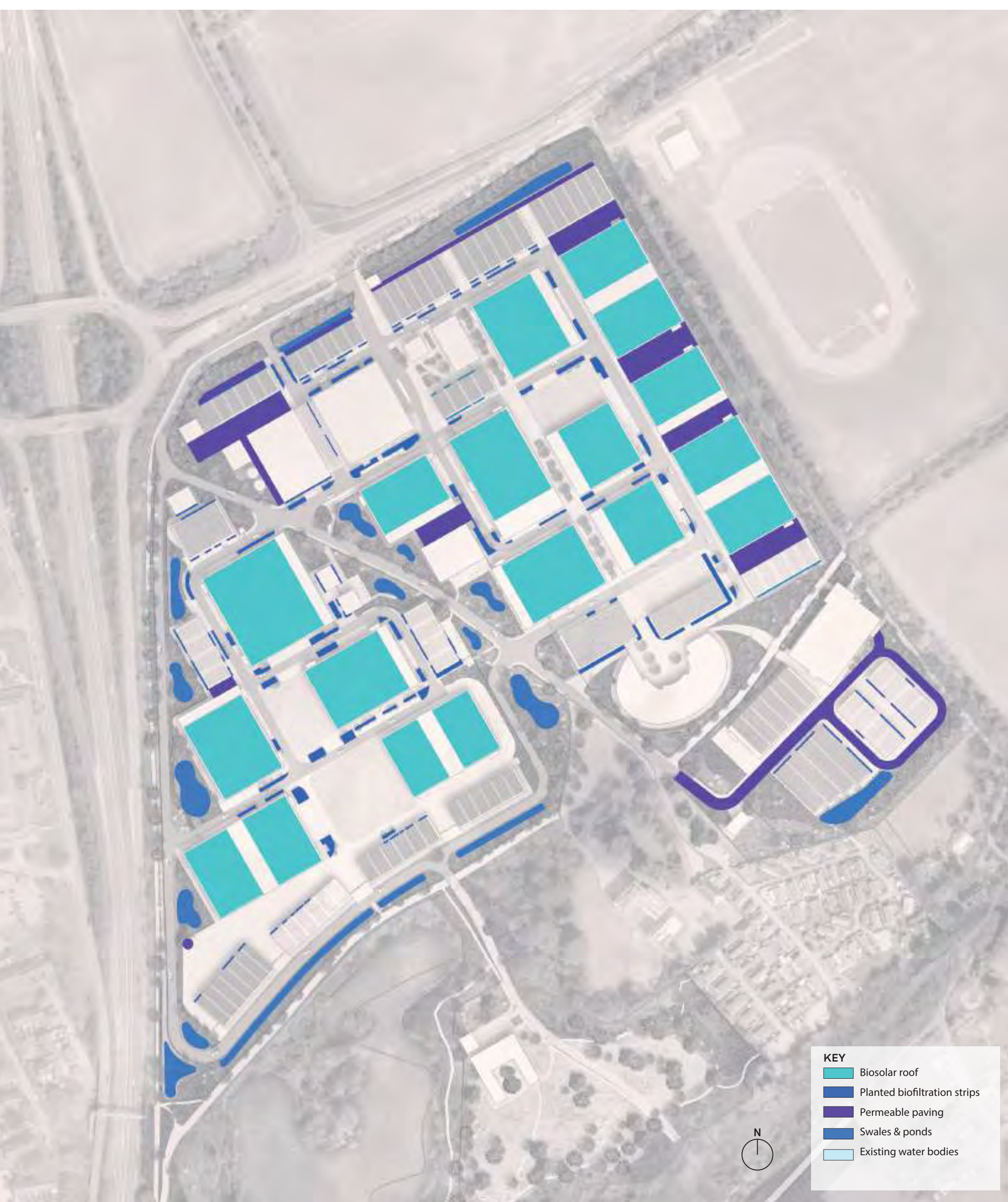
Diagram indicating water attenuation strategy
